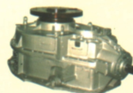
Coal Pulverising Mill Gearbox
